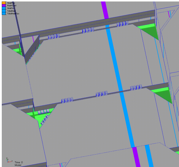
Figure 4: Thermal model with boundary conditions (colored stripes), detail with cells, interconnectors and Kapton layer (green)
