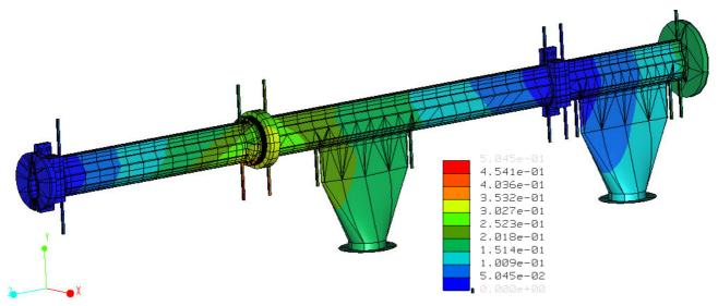
Figure 5: Displacements in all directions of vaccum chambers 1 and 2 due to the temperature loads;, maximum displacement of the chamber walls is 0.35 mm
