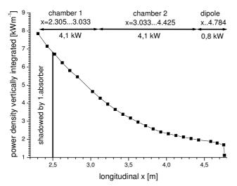
Figure 3: Heat load on inner vacuum chamber walls
