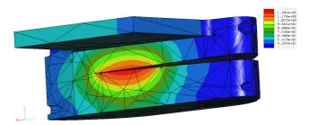
Figure 6: 2<sup>nd</sup> absorber: Temperature distribution on inward side, that defines the inner vertical aperture of the photon beam; 6 kW radiation impinges from right side, upper plate is used for mounting purposes
